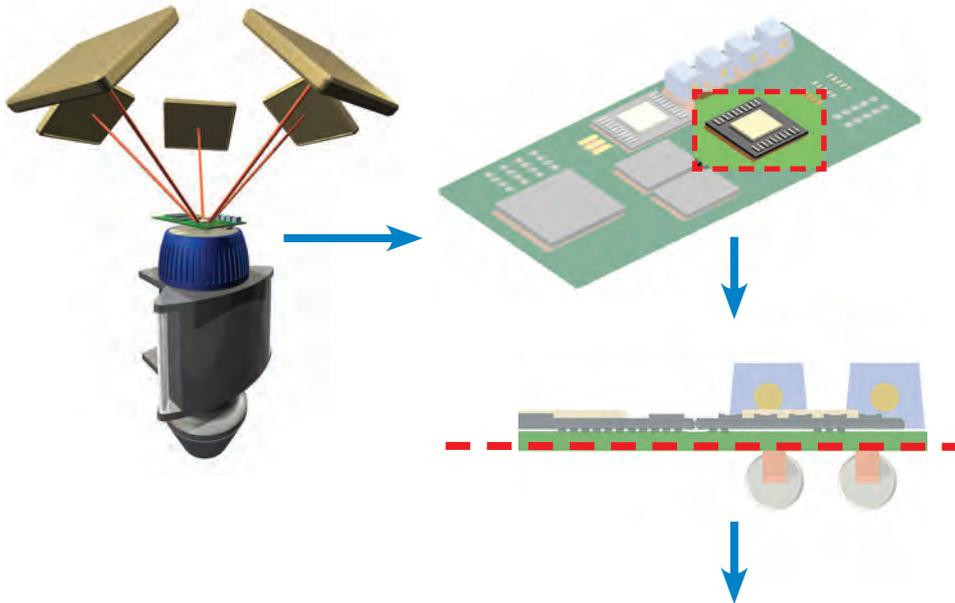
X-Plane™ is quick, simple and easy to use. The board is placed in the Nordson DAGE X-ray inspection system and X-ray images are taken 360° around the region of interest. Once image acquisition is complete, proprietary, and patent applied for, tomosynthesis produces a detailed 3D model which can be sliced and analysed in any plane using the supplied X-Plane™ Viewer.
